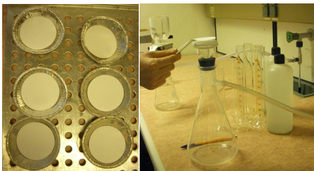
Figure 15: The picture to the left shows the GF/C filters in the aluminum dishes before filtration. The picture to the right shows the setup of the filtration system.
