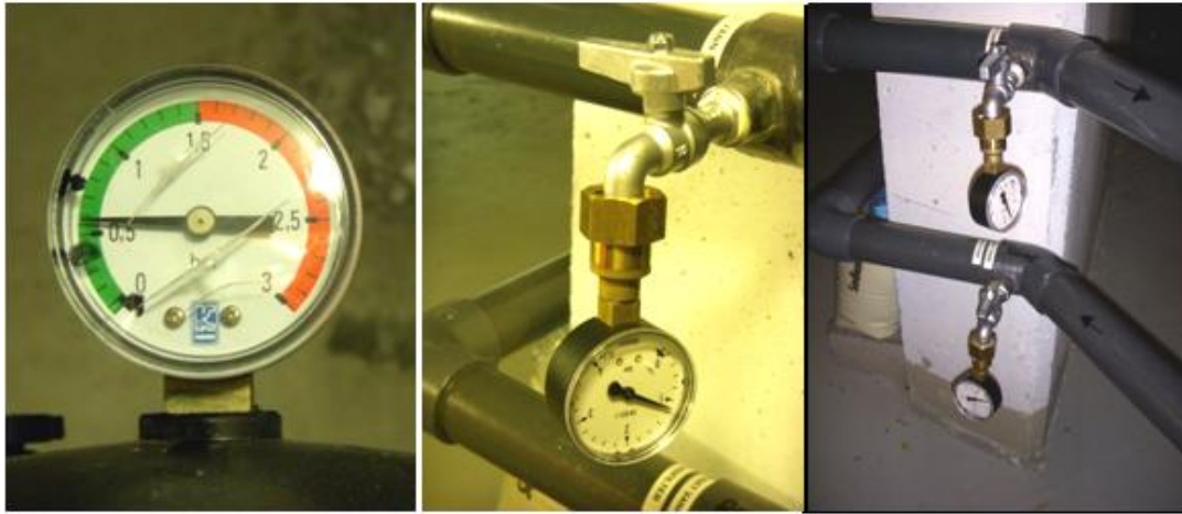
Figure 12: Experimental setup of the manometers, for the pressure measurements. The picture to the left shows the manometer on the top of the glass filter.
