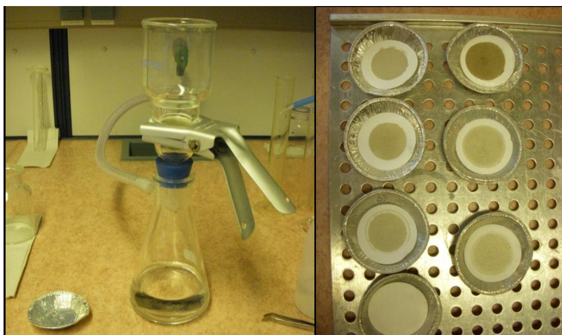
Figure 17: The picture to the left show the filtration setup after filtration of the water samples. The picture to the right shows the GF/C filter after filtration of the water samples, before drying.
