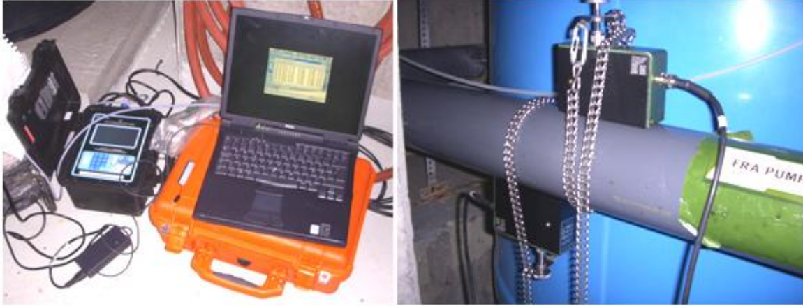
Figure 10: Experimental setup of the flow rate measurement on the sand filter. The picture to the left shows the data logger while the picture to the right shows the transducer and reflector installed at the water pipe.
